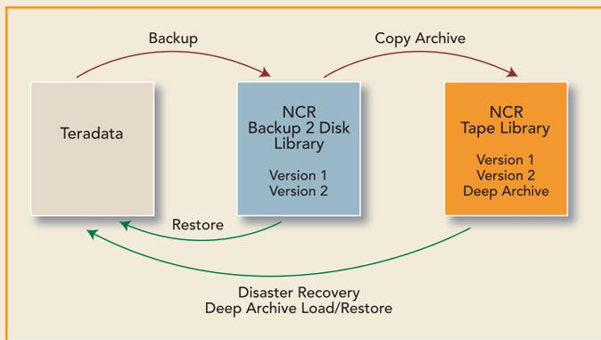
The two-tier disk-to-tape backup infrastructure utilizes BAR servers that are connected to an NCR Backup 2 Disk Library and an NCR Tape Library, enabling the Teradata Database to back up to disk in this LAN-based architecture. The BAR servers manage archiving data from the NCR Backup 2 Disk Library to the NCR Tape Library without requiring Teradata Database resources.
